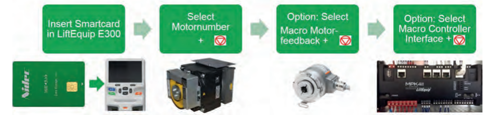
Figure 11: Commissioning and parameterisation
