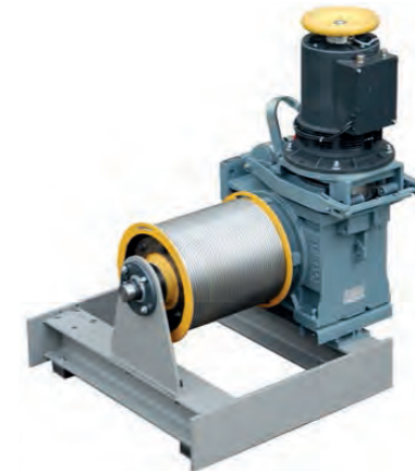
Figure 6: Geared unit TW130 with drum and traction sheave with outer bearing on frame
